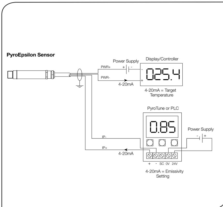
The PyroEpsilon Series is a range of high quality, low cost, compact sensors which measure the temperature of inaccessible or moving objects and materials. They measure temperatures from  $-20^{\circ}\text{C}$  to  $500^{\circ}\text{C}$ , accurately and consistently, with an outstanding response time of 240 ms.
