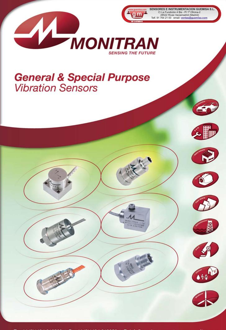
Monitran's general purpose accelerometers fall into two categories: those for vibration analysis, which have AC outputs and are suitable for use with hand-held and on-line vibration analysers; and those for machine protection, which have DC outputs and are ideal for direct input to a PLC or other industrial controller.
