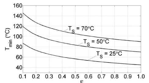
Graph showing the minimum measurable object temperature (T<sub>min</sub>), determined by surface emissivity (ε) and sensor temperature (T<sub>s</sub>).
