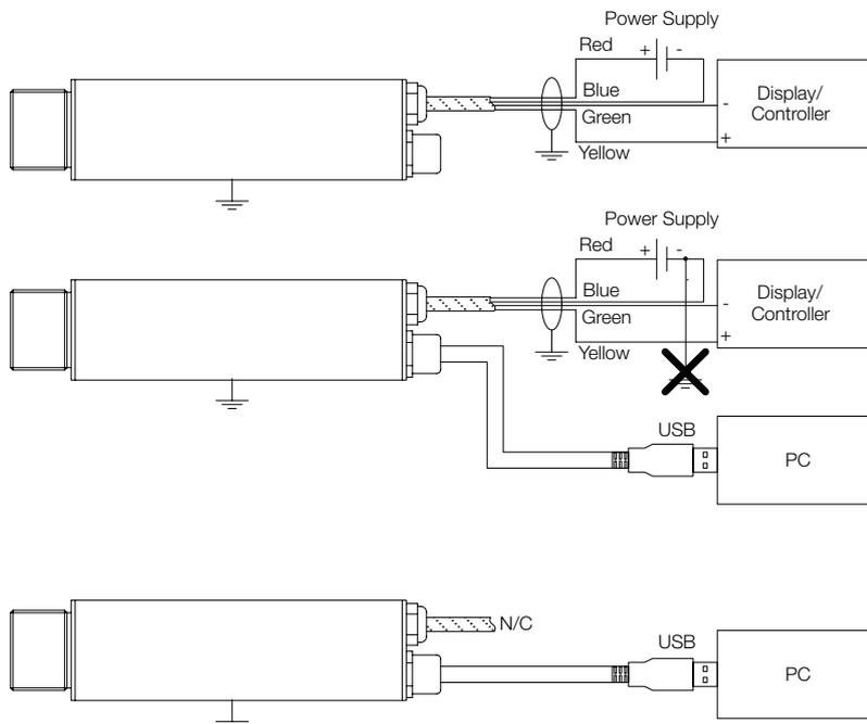
**Note:** The sensor must be grounded at only one point, either the cable shield or the sensor housing.
